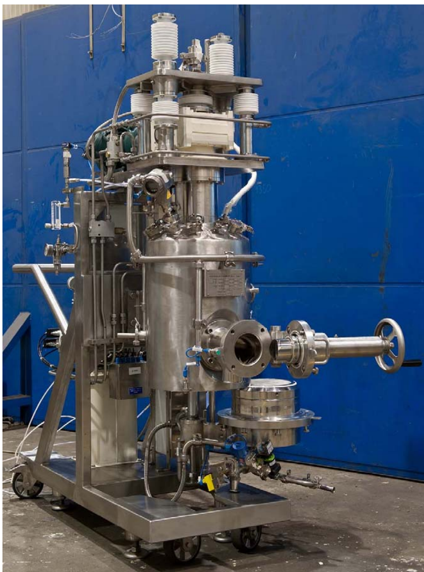
Pressofiltro® PF 10 with 0.045 m 2 filtration area
