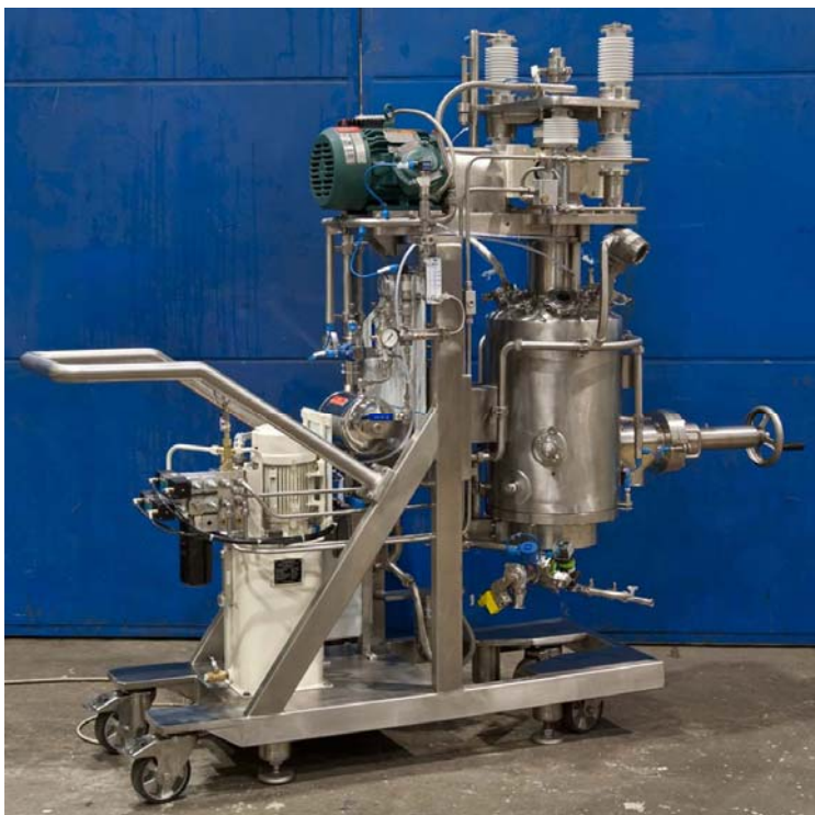
Pressofiltro® PF 10 0.045 m 2 filtration area
