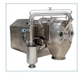
**HEINKEL** developed the inverting filter centrifuge in the early 1970s and can now look back on many years of experience. At that time the technology for automated product discharge with no residual layer and gentle on the grain was new; it is now time-proven, accepted and highly regarded in all application areas of the chemical industry.
